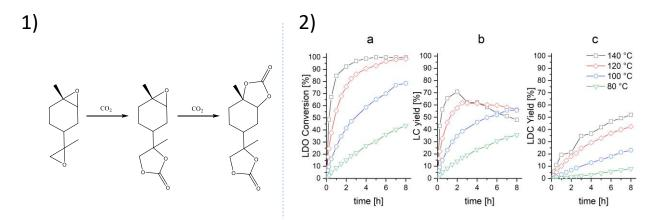
**Figure 1**: Reaction scheme of limonene dioxide carbonation (1). Temperature effect on the kinetics of limonene diepoxide carbonation (2).
