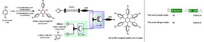
Figure 1. Optimized flow procedure for the synthesis of HABs.
