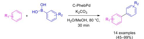
Figure 1: General scheme of Suzuki-Miyaura reactions catalysed by C-PhebPd.
