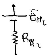
$$E_{H2} = \frac{E_H/R_{eq} + E_2/R_2}{\frac{1}{R_{eq}} + \frac{1}{R_2}} = \frac{25/12 + \frac{3}{2}}{\frac{1}{12} + \frac{1}{2}} = 5,29 \text{ V}$$
