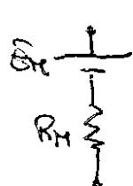
$$E_H = \frac{E_2/R_2 + T}{\frac{1}{R_2}} = \frac{10/5 + 3}{\frac{1}{5}} = 25 \text{ V}$$
