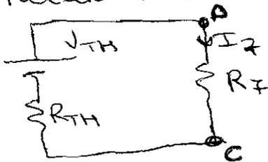
$$I_7 = \frac{V_{TH}}{R_{TH} + R_7} = -1,43 A$$
