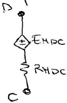
$$E_{HDC} = \frac{E_{HAC}}{R_{HAC} + R_6} - I' + \frac{E_3}{R_3} = -5 + 0,7I_3 [V]$$
