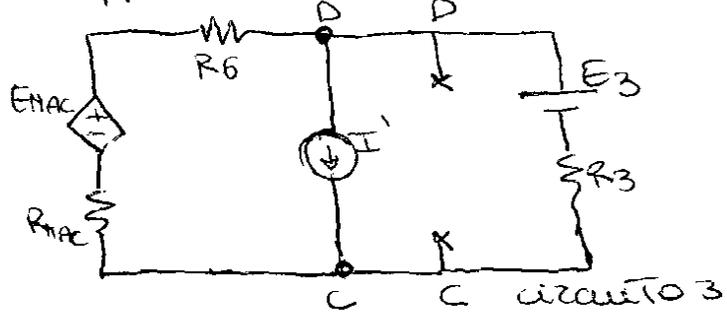
$$E_{HAC} = \frac{E_{HAB}}{R_{HAB} + R_5} + \frac{E_2}{R_2} = 3,34 + 0,84I_3$$
