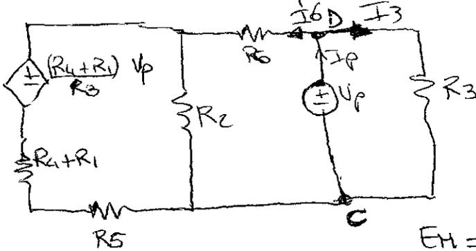
$$I_p = I_6 + I_3 = I_6 + \frac{V_p}{R_3} \quad (2)$$
