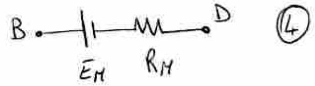
$$E_M = \frac{\alpha I / R_5}{\frac{1}{R_5} + \frac{1}{R_{34}} + \frac{1}{R_M^*}} =$$
