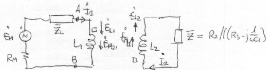
$$\dot{E}_M = \frac{\dot{E}_1 + \dot{E}_2}{\frac{1}{R_1}} \quad R_M = R_1 \quad \bar{Z}_L = R_L + j\omega L_L$$
