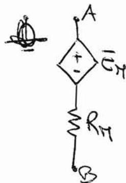
$$E_H = \frac{\frac{E_1}{(R_1+R_2)} + \alpha I}{\frac{1}{R_1+R_2} + \frac{1}{R_2+R_3}} = \frac{\frac{5}{3} + 2I}{\frac{1}{3} + \frac{1}{8}} = (3,63 + 4,36I) V$$
