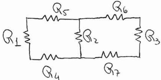
$$R_1 = R_2 = R_3 = R_4 = R_5 = \frac{l}{\mu \cdot \mu_r \cdot S} = \frac{10 \cdot 10^{-2}}{4 \pi \cdot 10^{-7} \cdot 10^3 \cdot 10 \cdot 10^{-6}} = 7,96 \cdot 10^4 \text{ H}^{-1}$$
