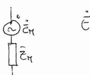
$$\dot{E}_H = \frac{\dot{E}_L - \dot{E}_2}{\frac{1}{\dot{Z}_1} + \frac{1}{\dot{Z}_2}} = \frac{2,5 + j4,33}{\frac{1}{5+j} + \frac{1}{3+j^2}} = -1,74 + j2,40 \text{ V}$$
