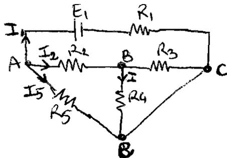
$$R_{34} = R_3 \parallel R_4$$
