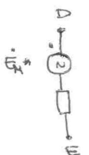
$$\dot{E}_M^* = \frac{\frac{\dot{E}_M}{R_M + R} + \alpha V_{AB}}{\frac{1}{R_M + R} + \frac{1}{\bar{Z}_P}}$$
