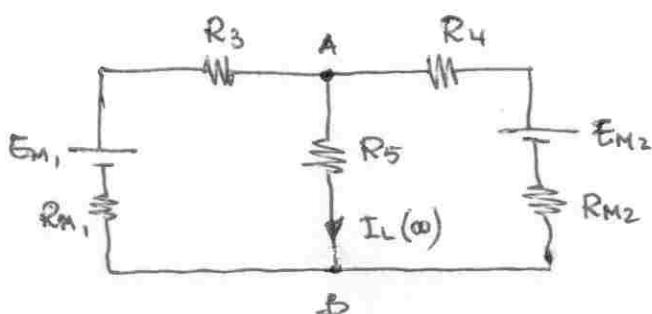
$$EM_1 = \frac{\frac{E_1}{R_1} - I}{\frac{1}{R_1}} \quad RM_1 = R_1$$
