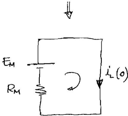
$$E_M = \frac{\frac{E_1}{R_1} - J - \frac{E_2}{R_2}}{\frac{1}{R_1} + \frac{1}{R_3} + \frac{1}{R_2} + \frac{1}{R_5}} = -2,87 \text{ V}$$
