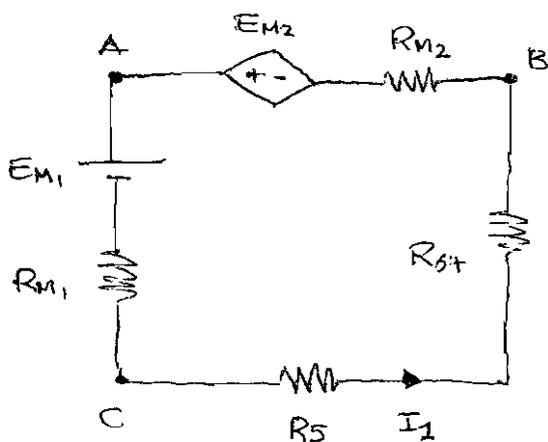
$$E_{M1} = \frac{\frac{E_1}{R_1} - I}{\frac{1}{R_2}}; \quad R_{M1} = R_1;$$
