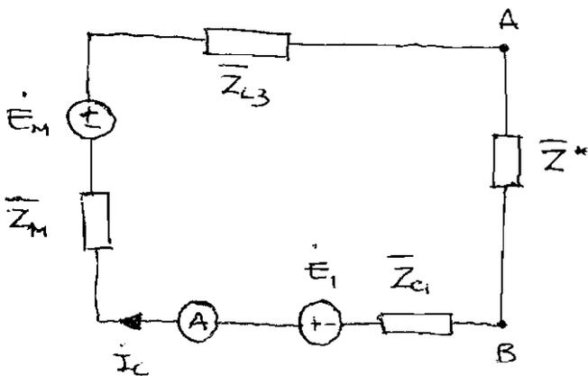
$$\text{con } \bar{Z}^* = \frac{\bar{Z}_{R1} \cdot (\bar{Z}_{R3} + \bar{Z}_{L4})}{\bar{Z}_{R1} + \bar{Z}_{R3} + \bar{Z}_{L4}}$$
