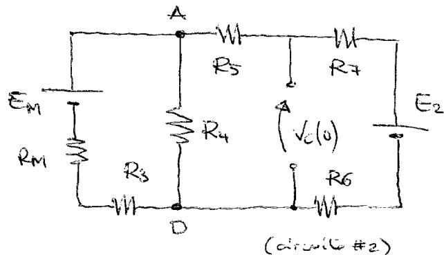
$$E_M = \frac{\frac{E_1}{R_1} - I_1}{\frac{1}{R_1}} = 7V$$
