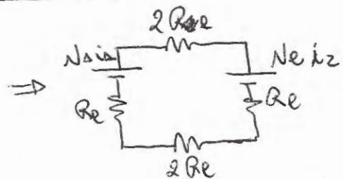
$$R_p = \frac{l}{\mu_0 N_p S} \Rightarrow R_{eq} = R_p + 2R_s + 2R_p + R_p = 6R_p$$
