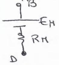
$$E_H = \frac{\left( \frac{E_{H1} + E_{H2}}{R_{H1} + R_{H2}} \right) + \frac{E_{H3}}{R_6 + R_7}}{\frac{1}{R_{H1} + R_{H2}} + \frac{1}{R_5} + \frac{1}{R_6 + R_7}}$$
