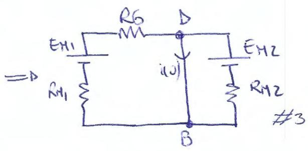
$$E_{M1} = \frac{E_1/R_1}{\frac{1}{R_1} + \frac{1}{R_3}}$$
