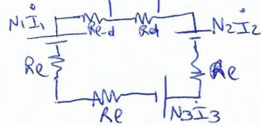
$$R_{eq1} = R_{eq2} = R_{eq3} = R_{eq} = 3R_e + R_{e-d} + R_d$$
