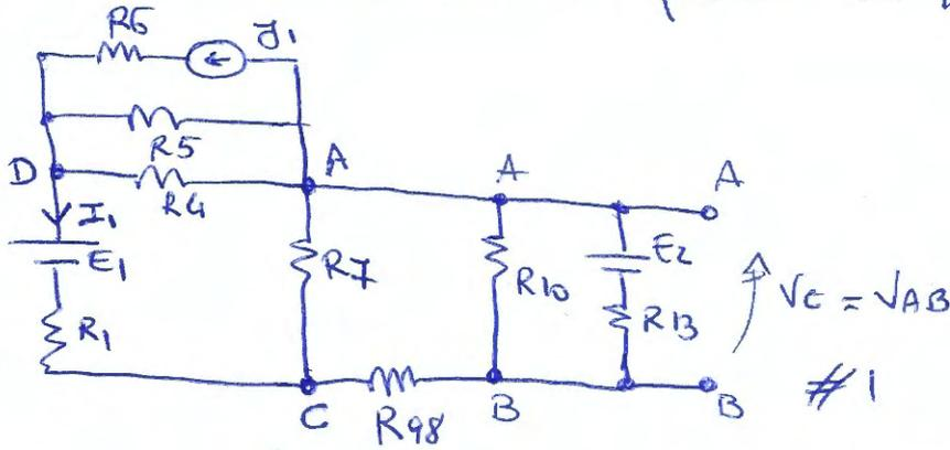
$$R_{98} = \frac{R_9 \cdot R_8}{R_9 + R_8}$$
