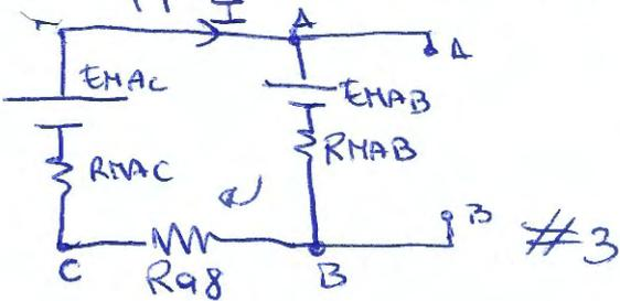
$$E_{MAC} = \frac{(E_1 - E_{MDA})}{\frac{1}{R_1 + R_{MDA}} + \frac{1}{R_7}}$$
