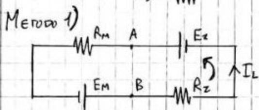
$$R_M = \left( \frac{1}{R_4} + \frac{1}{R_3} \right)^{-1} = 5.33 \Omega$$
