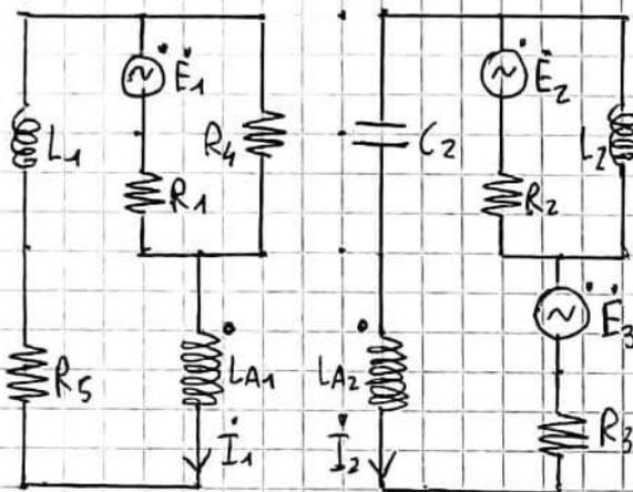
$R_{M1} = \left( \frac{1}{R_1} + \frac{1}{R_4} \right)^{-1} = 2.31 \Omega$
