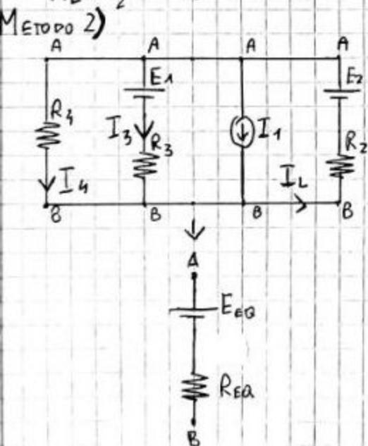
$$R_{eq} = \left( \frac{1}{R_4} + \frac{1}{R_3} + \frac{1}{R_2} \right)^{-1} = 3.20 \Omega$$
