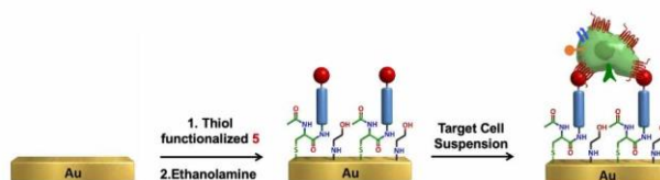
Figure 1. Schematic illustration of the SPR-POF platform functionalization and target cell capture principle.
