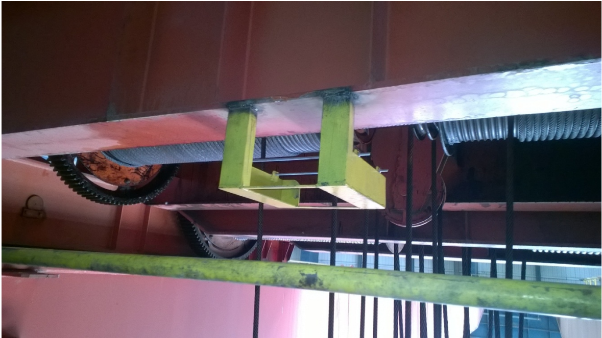
Figure 21. Metallic support for the prototype positioning.
