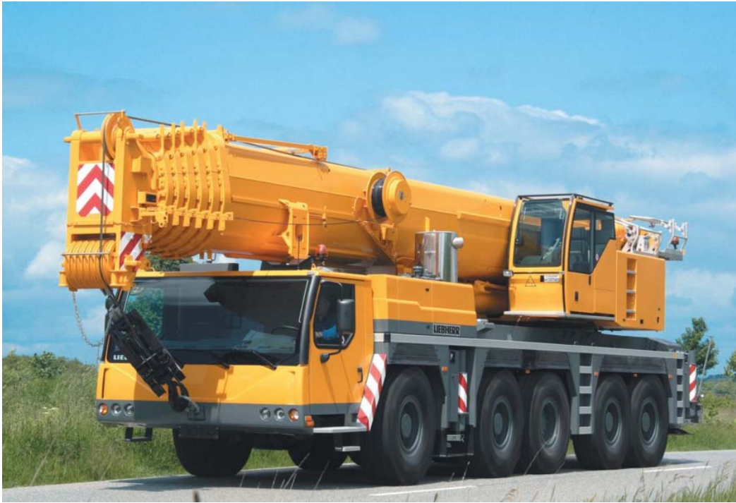
Figure 1. Selected crane from the Lorefice & Ponzio Company (Liebherr LTM 1200-5.1), source [17].
