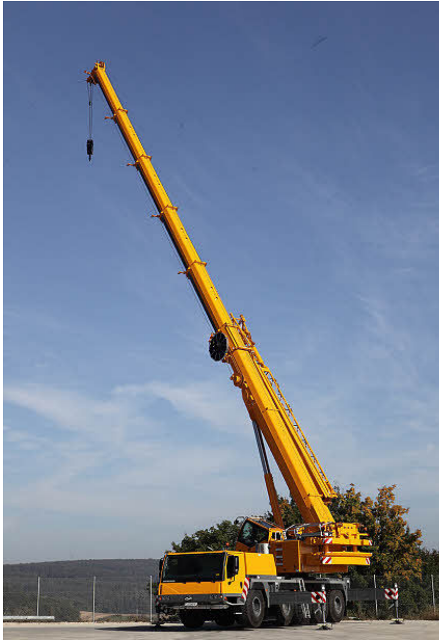
Figure 3. Maximum extension of the telescopic boom of a crane Liebherr LTM 1200-5.1.
